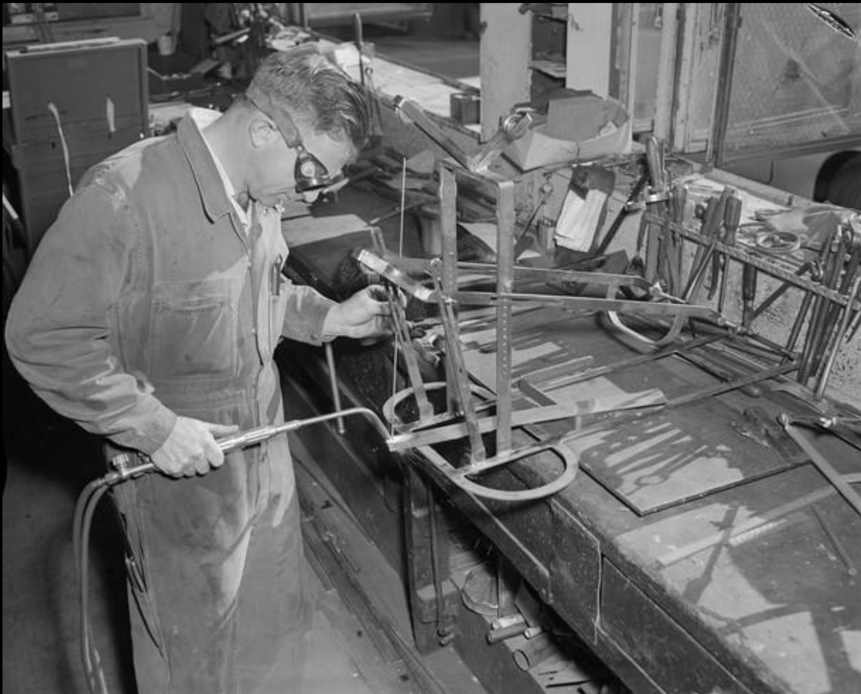
A male manufacturing worker welding part of a metal leg elevation device for above a hospital bed in a workshop at the Royal Children's Hospital
