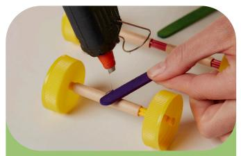
Glue the popsicle sticks to the straws, making a triangle shape between the front and rear axle.
